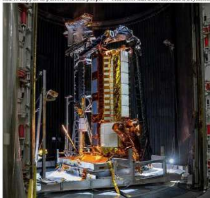
A view of NISAR before the chamber door was closed ahead of its thermal vacuum testing at the Jet Propulsion Laboratory, California, January 4, 2022. NASA
